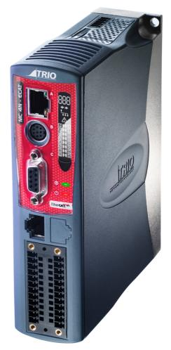
The MC4N-ECAT has one built in RS232 port and one built in duplex RS485 channel for simple factory communication systems. Either the RS232 port or the RS485 port may be configured to run the Modbus or Hostlink protocol for PLC or HMI interfacing.
