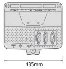
Ethernet and serial connections. A slot is provided for the optional Micro SD card.
