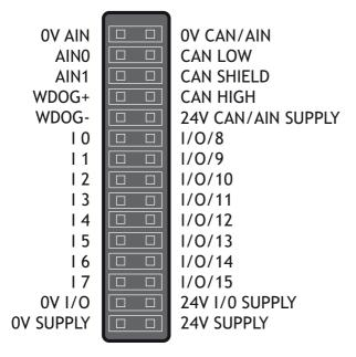
The MC664 is powered entirely via the 24V d.c.supply connections. The unit uses internal DC-DC converters to generate independent 5V logic supply, the encoder/serial 5V supply and other internal power supplies. I/O, analogue and CANbus circuits are isolated from the main 24V power input and must be powered separately. For example; it is often necessary to power the CANbus network remotely via the CANbus cable.
